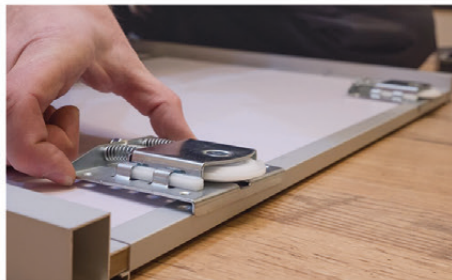
12. Place the wheels into position at the bottom of the frame
