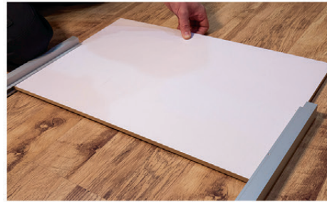
7. Lay the first door frame out on a soft floor surface to avoid scratching the panels or frame
